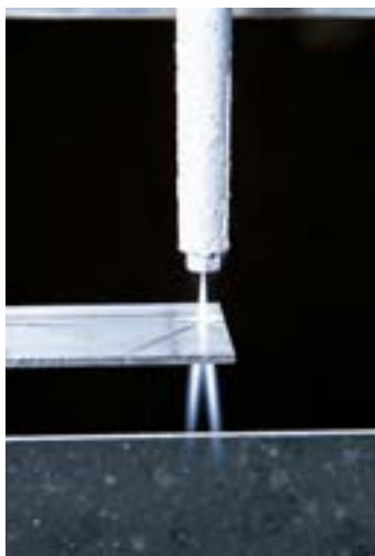
LIKE A KNIFE through warm butter, a high-pressure jet of liquid nitrogen hews through hard materials, then disappears into thin air.
