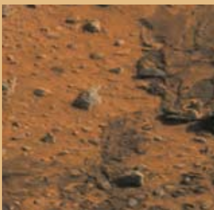
DRAG MARKS , left by the air bags as they were retracted, indicate a cohesive soil—perhaps electrostatically charged dust or a weakly cemented “duricrust” like that seen by Viking.
