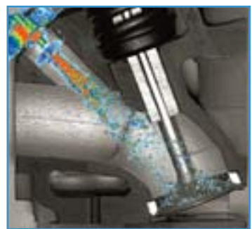
ATOMIZED GASOLINE (colorized) emitted by a fuel injector hits an air-intake valve as it begins to open, in an experiment at Sandia National Laboratories.
