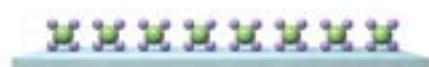
2 Molecules of ZrCl_4 adhere to the surface but not to one another.
