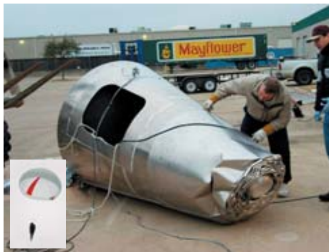
CRUSHABLE NOSE CONE will cushion the landing when Armadillo Aerospace's Black Armadillo spacecraft returns from its planned suborbital flight. A subscale model is shown parachuting down in a drop test (inset). After the experiment, engineers inspected how the model's nose structure collapsed to absorb the forces of impact.
