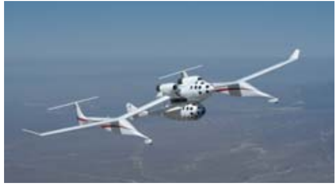
WHITE KNIGHT , the mother ship for SpaceShipOne (seen attached below the large airplane's fuselage), will release the three-seat spacecraft at about 50,000 feet. Scaled Composites's rocket will then climb to suborbital altitude.
