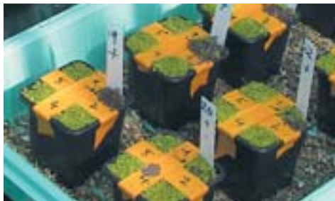
RED WEED BAD: Explosives in soil cause plants to redden (in each pot, quadrants to right of label “1”).
