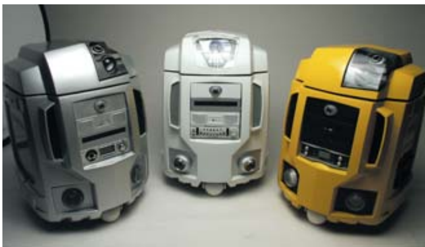
PC-BOT PLATFORM can be customized with PC accessories, allowing the basic 912 model (left) to be transformed into a DVD-playing 912 MP3 (center) or a 912 HMV security rover (right).
