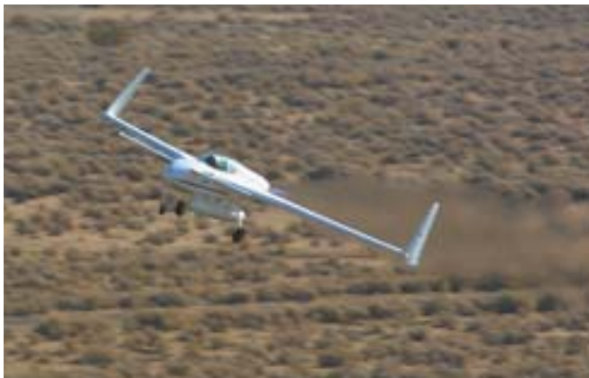
LONG-EZ SPORT PLANE was fitted with an experimental liquid-fueled rocket motor for aerial tests by engineers at XCOR Aerospace.
