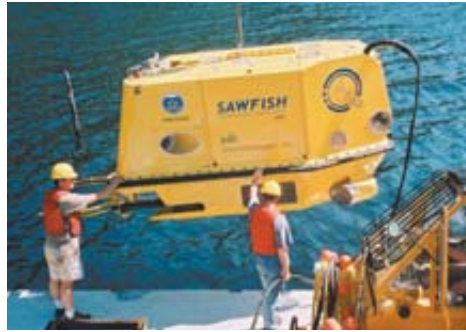
SAWFISH , operated by the Canadian firm Triton Logging, can dive at least 1,000 feet—as deep as any reservoir in the world.
