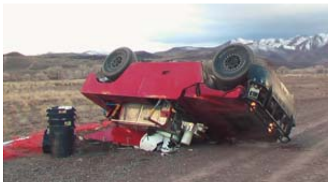
HEAD OVER WHEELS , the Sandstorm robot crashed in a test four days before the competition. A change of a single digit in its steering and speed control software caused the robot to go too fast on a turn.
