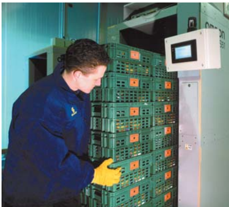
SMART PORTAL equipped with an RFID tag reader identifies and inventories an incoming shipment of foodstuffs stored in crates fitted with computerized smart labels. The high cost of RFID tags currently limits their use to labeling multicomponent loads of goods rather than individual items.
