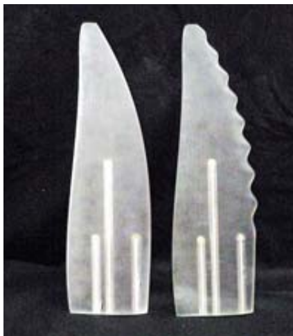
PECTORAL FLIPPER REPLICAS, with and without bumps, went fin to fin in wind-tunnel tests.
