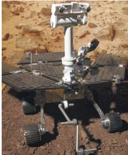
MODEL ROVER is displayed at Cornell University. Working duplicates enable maneuvers to be tested on Earth first.
