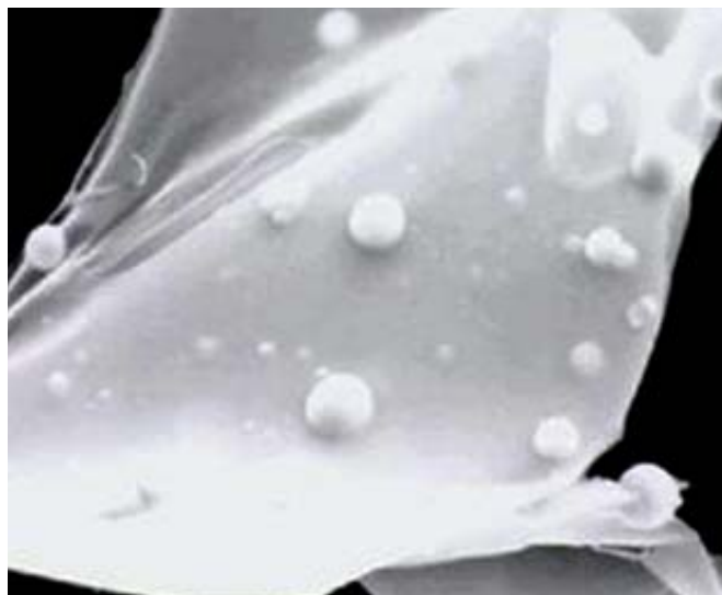
MICROSPHERES can be incorporated throughout a scaffold by mixing them into the alginate solution before freeze-drying. Only three microns in diameter, the microspheres accelerate blood vessel formation—without getting in the way—by steadily releasing growth factors.
