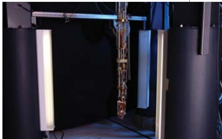
Microscope plus MRI detects the force of an electron's spin.
