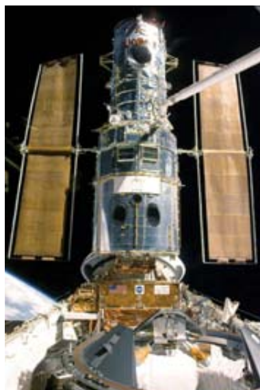
MANHANDLED: The Hubble Space Telescope is brought into the space shuttle’s cargo bay by its teleoperated arm during the 1999 servicing mission.
