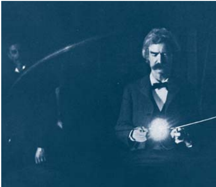
MARK TWAIN (Samuel Clemens) demonstrates the wireless transmission of power. A large resonating coil (not visible) has induced a high-voltage current in the wire loop he holds. The current passed harmlessly through Twain's body yet caused the incandescent bulbs to glow. Tesla is seen (obscured at far left) operating the apparatus's controls.
