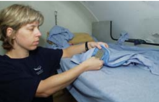
SILVER-LACED BEDSHEETS , T-shirts and other fabrics, which resist microbial growth, were tested in NASA's Aquarius habitat.
