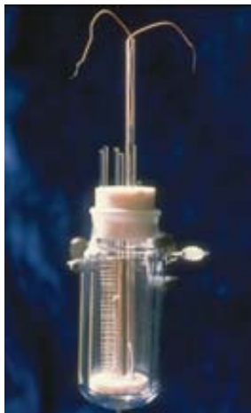
COLD FUSION allegedly occurs in a jar of heavy water with electrodes.
