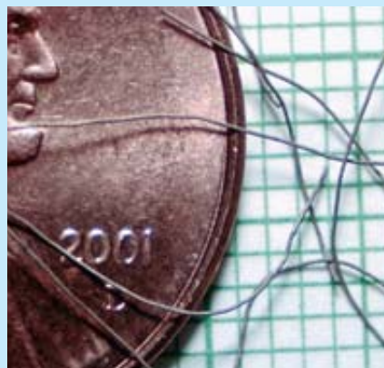
WIRES were made by reacting magnesium vapor and boron filaments.
