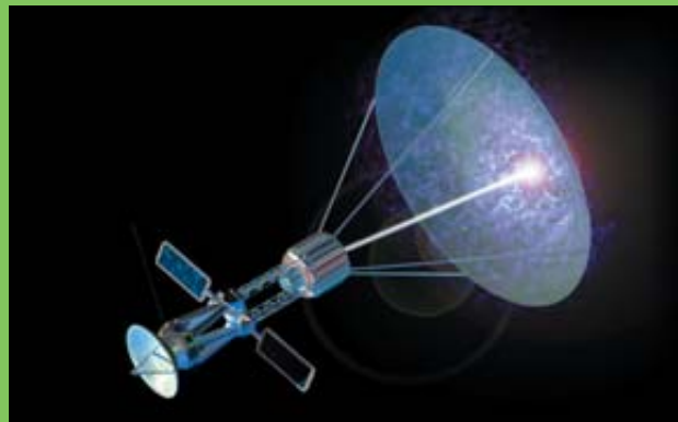
PROPOSED ANTIMATTER PROPULSION system uses antimatter pellets to trigger fission explosions on a uranium-coated sail.
