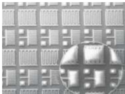
INDELIBLE IMAGE of a microscopic bubble gets imprinted on a wafer during immersion lithography, compromising the integrity of electrical circuits.
