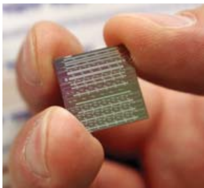
LIGHT WORK: Eight lasers constructed from inexpensive silicon reside in this chip made by Intel. The coherent light beams could lead to ultrafast computer circuitry that transmits data optically.
