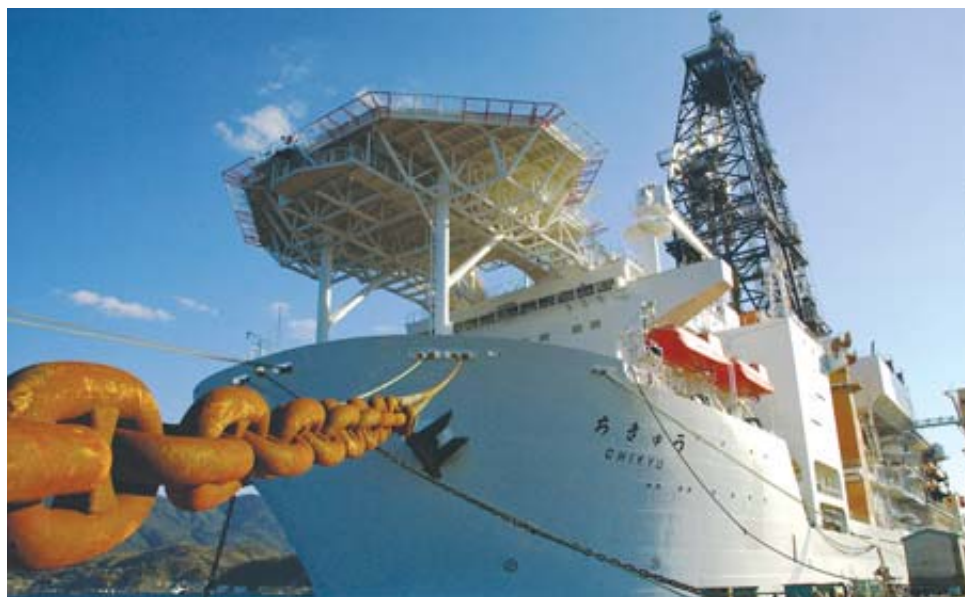
HEAVY DUTY: Deep-sea drilling vessel Chikyu , designed to penetrate through kilometers of rock to the earth's mantle, undergoes final outfitting at Mitsubishi Heavy Industries's shipyard in Nagasaki.
