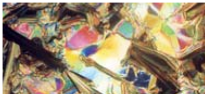
An organic film of phenylene vinylene molecules self-assembles into well-ordered layers that control charge flow.
