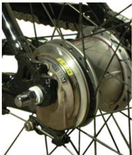
PLASTIC ENCLOSURE (top) contains the computer chip that selects the gears, which are inside a hub on the bike's rear axle (bottom).
