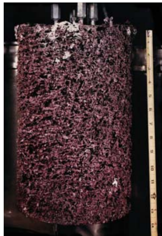
EXTRACTED URANIUM and actinide elements from spent thermal-reactor fuel are plated out on the cathode of an electrorefiner during the pyroprocessing procedure. After further processing, the metallic fuel can be burned in fast-neutron reactors.
