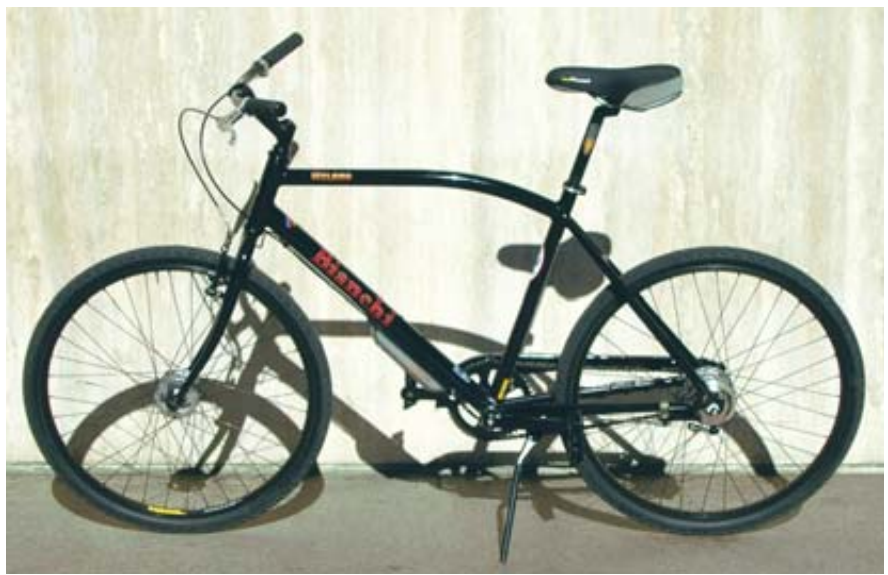
FREEWHEELING: No shift levers are on the handlebars of this Bianchi Milano bicycle. Instead an automatic transmission system senses acceleration and does all the gearshifting.
