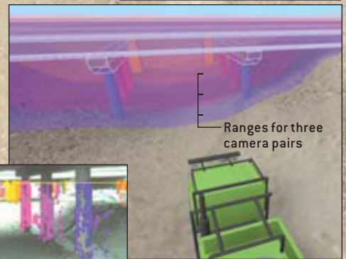
Terramax might first detect the pillars of an underpass with its long-range stereo cameras ( orange zone above ). As the vehicle slows, it will switch to medium- and then short-range camera pairs to make certain it notices all the obstacles in its video scene ( inset ).
