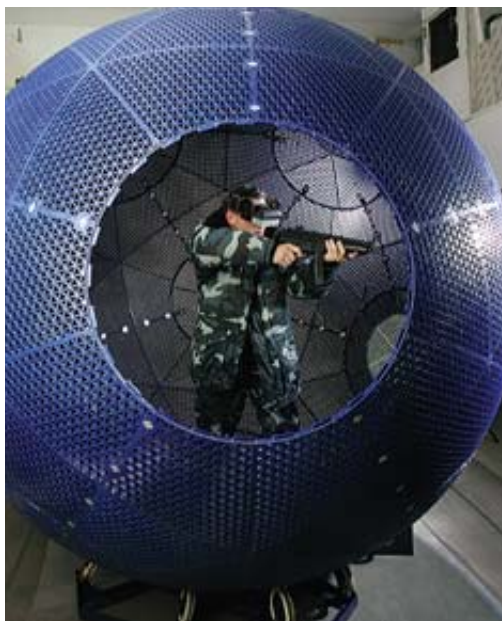
VIRTUSPHERE rotates in place as the user inside moves about. From the sphere's motions, a computer calculates the user's path in the simulated world.
