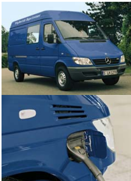
PLUG-IN HYBRID TECHNOLOGY from a major automaker debuted in 2005 with the rollout of the Mercedes-Benz Hybrid Sprinter Van prototype (top). A door opens to reveal the electrical socket for connecting the battery to a power source and charging it overnight (bottom).
