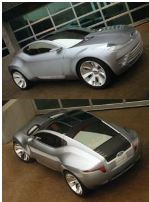
DIESEL-ELECTRIC HYBRIDS, such as this Ford Reflex concept car, can achieve even better mileage than gasoline-electric vehicles. The Reflex prototype is expected to deliver up to 65 miles per gallon of diesel fuel and also features solar panels in the headlights and taillights to generate auxiliary power for the battery.
