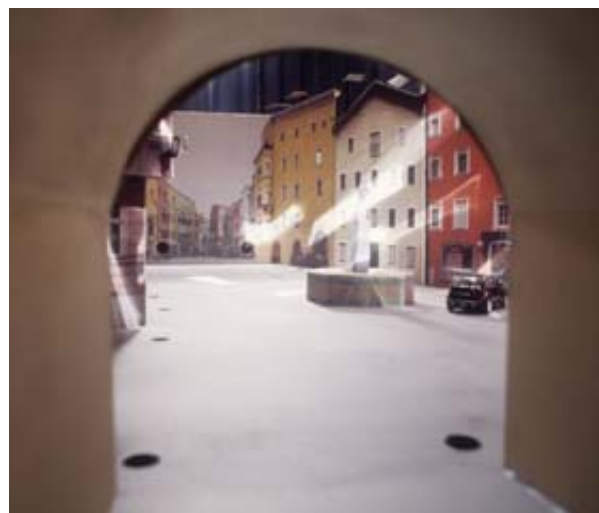
HERE COMES THE SUN: Scale model of a street in Rattenberg, an Alpine village that gets no winter sun, shows what residents will see when reflectors called heliostats bounce light into town. Bartenbach Light Laboratory plans to install the heliostats this summer.
