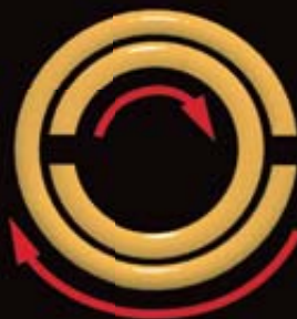
Circular currents flow in split-ring resonators (SRRs).
