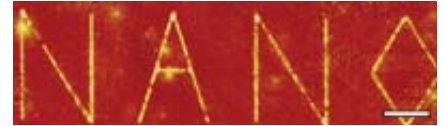
a 35-nanometer layer of silver in place ( right ). Scale bar is 2,000 nanometers long. With the superlens, the resolution is finer than the 365-nanometer wavelength of the light used.
