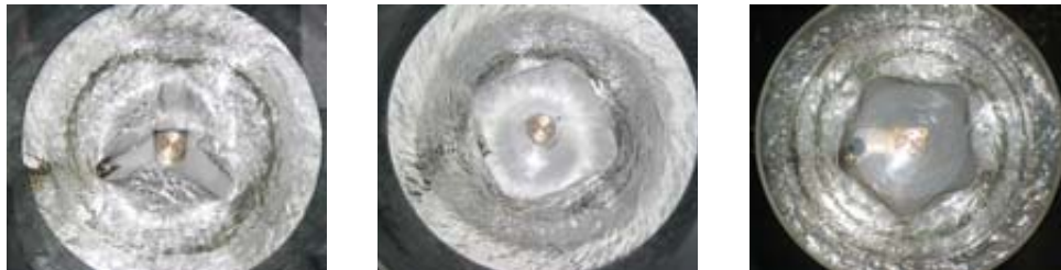
SPIN CYCLE: Water adopts trefoil, square and pentagonal shapes depending on the rotational speed.
