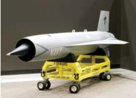
FAST AND FURIOUS: RATTLRS cruise missile, as shown in this mock-up, could set speed records, thanks to a movable air-inlet spike and a novel engine.
