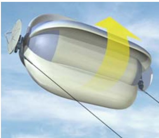
▲ Like a spinning blimp, a helium-filled rotor would catch the wind in fabric scoops, turning generators attached to tethers, which would then conduct the electricity to a transformer on the ground.
