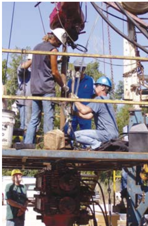
BURIAL SERVICE: Carbon dioxide in a supercritical fluid state is pumped into the Frio Formation in Texas as a test of underground carbon storage.
