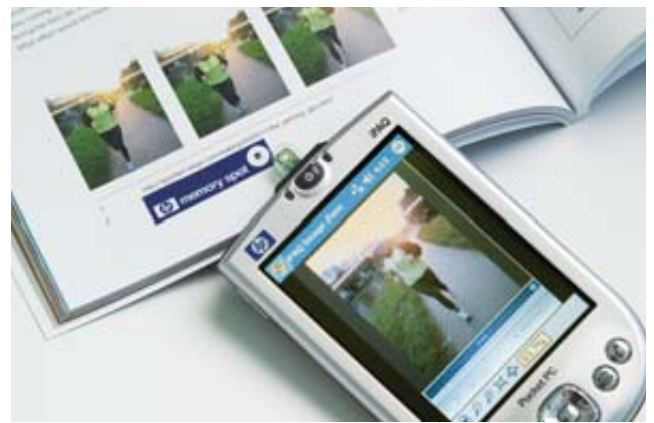
Memory Spot embedded in a book could provide supplemental text, images and video to anyone with a portable reader.
