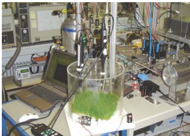
AUTHORS' EXPERIMENT detected minuscule quantities of methane produced by living vegetation ( rye grass in photograph ).
