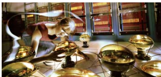
BOON FOR NEUTRINOS: A researcher examines the photomultiplier tubes that detect the flashes of light from neutrino interactions.
