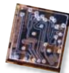
ACTUAL SIZE: The University of Michigan's influenza chip measures 1.5 by 1.6 centimeters.
