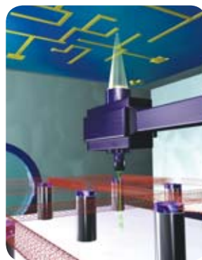
CARBON NANOTUBE NETWORK could be grown across pillars, then mapped and stamped onto an electronic circuit.
