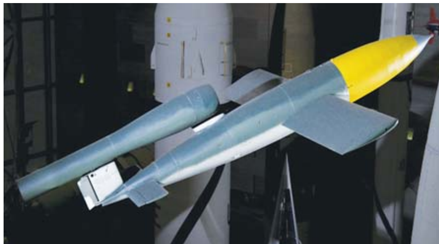
BUZZED: Germany's V-1 flying bomb relied on the pulse jet engine. Similar engines featuring much faster fuel combustion offer better performance and fuel efficiency.
