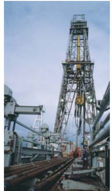
▲ DRILL RIG towering over the deck of the JOIDES Resolution lowered and raised the long drill pipe (foreground) that the author and his team sent to the seafloor to extract rock cores from seamounts.
