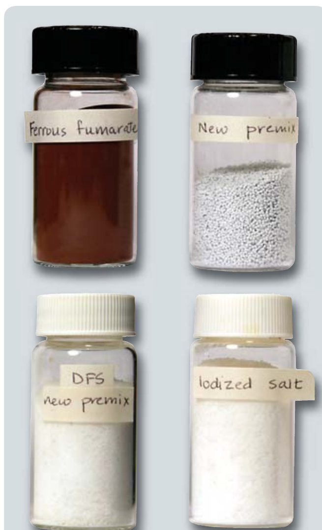
NOW WITH IRON: A key to making fortified salt acceptable to people is to ensure that the iron looks like salt. In the vials (clockwise from top left): iron particles; iron coated with titanium dioxide; iodized salt; and iodized salt mixed with the coated iron.
