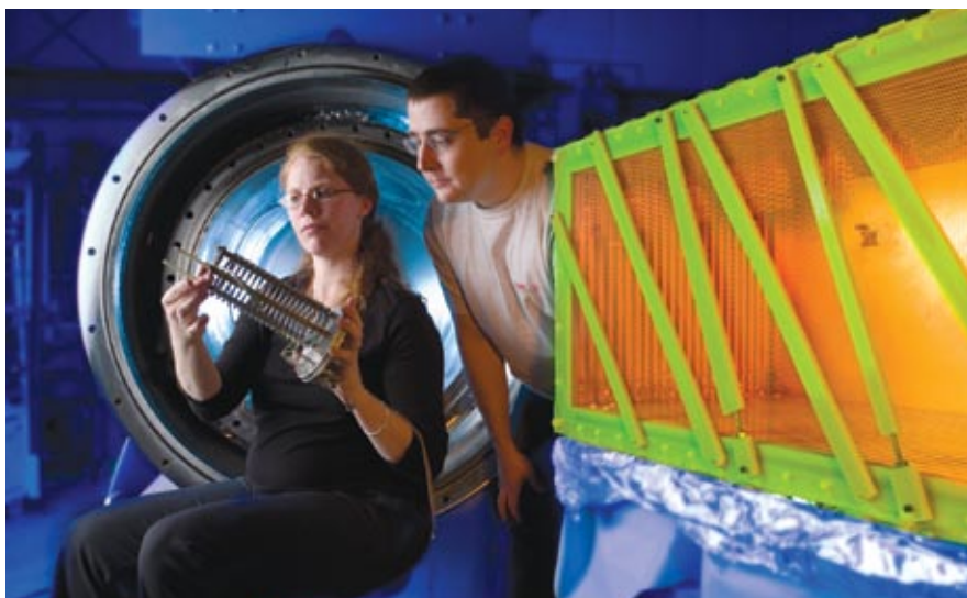
NEUTRINO HUNTERS Bonnie Fleming and Mitchell Soderberg inspect a prototype liquid-argon detector called ArgonNeUT that will pave the way for the MicroBooNE facility at Fermilab.
