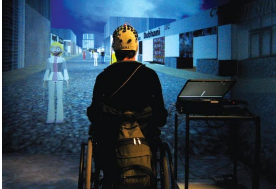
▲ QUADRIPLEGIC confined to a wheelchair can negotiate a virtual street using brain waves captured by an electrode cap.
