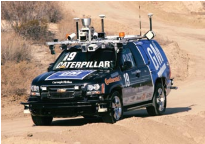
“BOSS” ROBOTIC VEHICLE (left), which won last year’s DARPA Urban Challenge autonomous vehicle competition, is the forerunner of future driverless cars and trucks that could be available in a decade. Such automated vehicles will be capable of “platooning,” or riding in close
