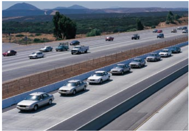
formation without driver intervention, as was demonstrated several years ago on a San Diego freeway (right). These kinds of “intelligent highway” technologies would allow vehicles to save space and limit accidents on the nation’s increasingly traffic-bound roads.
