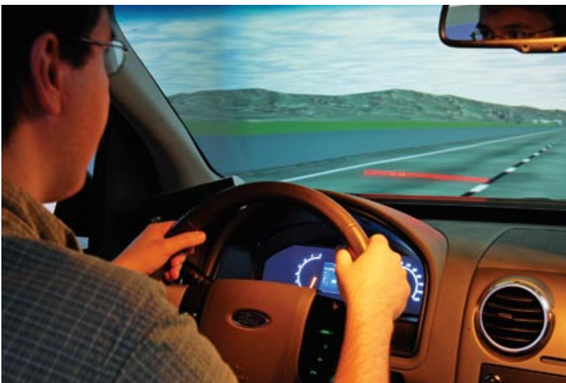
COLLISION WARNING , the red light strip reflected on the windshield in the left photograph, warns of a potentially hazardous obstacle in the roadway ahead during a “drive” in a Ford virtual-reality simulator. The navigation screen in the right photograph is linked to Honda’s new multiview camera system and displays a wide-angle, wraparound view from the back and rear sides of the vehicle.
