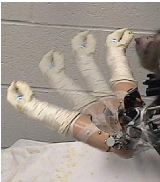
In this time-lapse image, a monkey with an implanted neuronal prosthesis uses thought alone to direct a motorized prosthetic arm to pick up food and deliver the food to its mouth.
