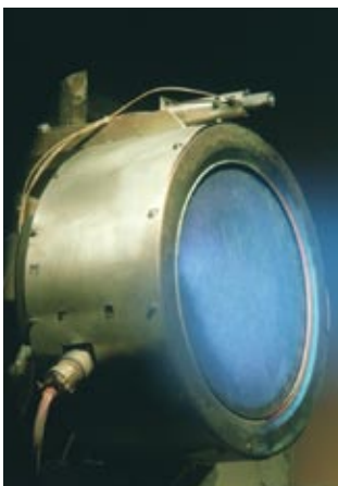
ION THRUSTER, which is 40 centimeters in diameter, was test-fired inside a laboratory vacuum chamber. Charged xenon atoms account for the blue color of the exhaust plume.
