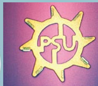
ROTARY MOTOR The same pair of chemical reactions moves protons and water around the teeth of this 100-micron-wide wheel, making it turn.
