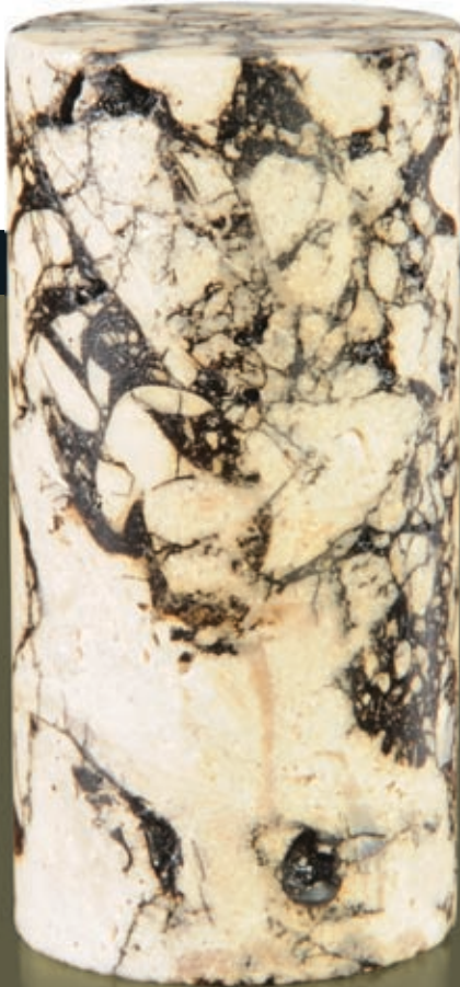
▲ Oil reservoirs are not underground lakes, but layers of oil-soaked porous rock. This five-centimeter-tall core comes from offshore fields near Sicily that are too expensive to develop with current technology. Its thick veins of oil feel solid to the touch, as if the white, carbonate rock were simply stained.
