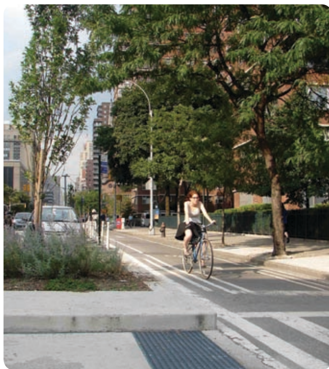
CYCLE TRACK, here along New York City’s Ninth Avenue, keeps bicyclists physically separated from motor vehicle traffic. Such designs make riding safer and could boost the number of women cyclists.
