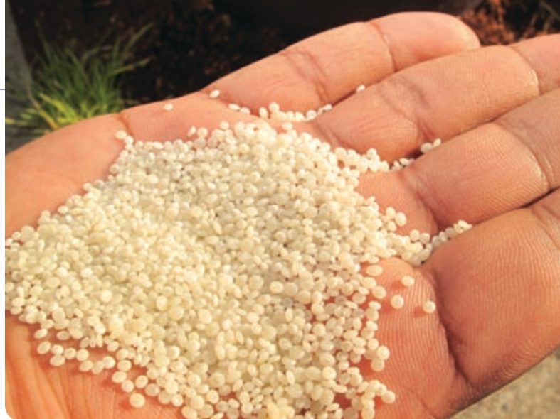
WASTEWATER WONDER: Ostara's Crystal Green, a slow-release fertilizer, incorporates phosphorus retrieved from sewage streams.
