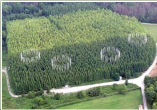
RINGS of vent pipes at the Free-Air CO 2 Enrichment experiment simulate heightened emissions by pumping the gas through trees.
