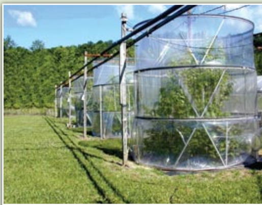
OPEN-TOP CHAMBERS at the Temperature Response and Adjustment Experiment warm saplings and small trees year-round.
