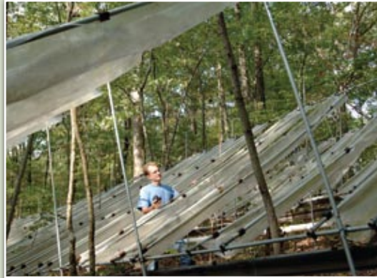
TROUGHS at the Throughfall Displacement Experiment simulate drought by preventing rainfall from reaching the ground.
