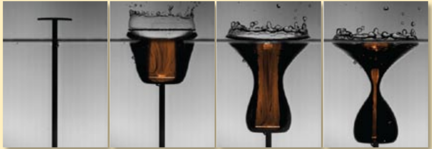
SUPERSONIC SPLASH: A disk pulled into water by a piston at a leisurely one meter per second creates a bubble that, as it collapses, briefly forces air to move faster than sound.
