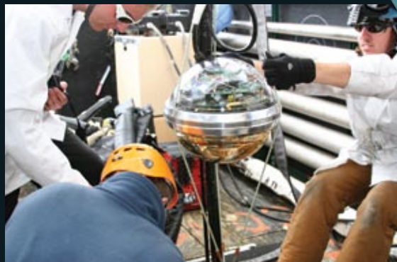
Scientists started work during the 2005–2006 southern summer and hope to wrap it up in the coming summer. They drill 2.5-km holes using hot water and lower the photodetectors on a cable.
