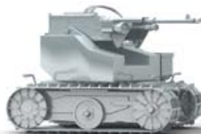
MAARS serves as a 160-kilogram machine gun-carrying and grenade-launching sentry and sniper.
