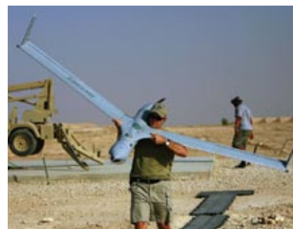
BRING YOUR OWN DRONE: The ScanEagle provided an airborne security camera for U.S. Marines in Iraq's Al Anbar province by hovering over remote tracts for hours on end.
