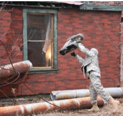
HELPING OUT: A soldier chucks a PackBot surveillance robot through a window so that its onboard video cameras can provide an inside view of the premises.
