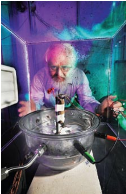
READY, SET, BLOW: In a battery safety test, Sandia researcher Peter Roth prepares to overcharge a lithium-ion cell until it explodes.
