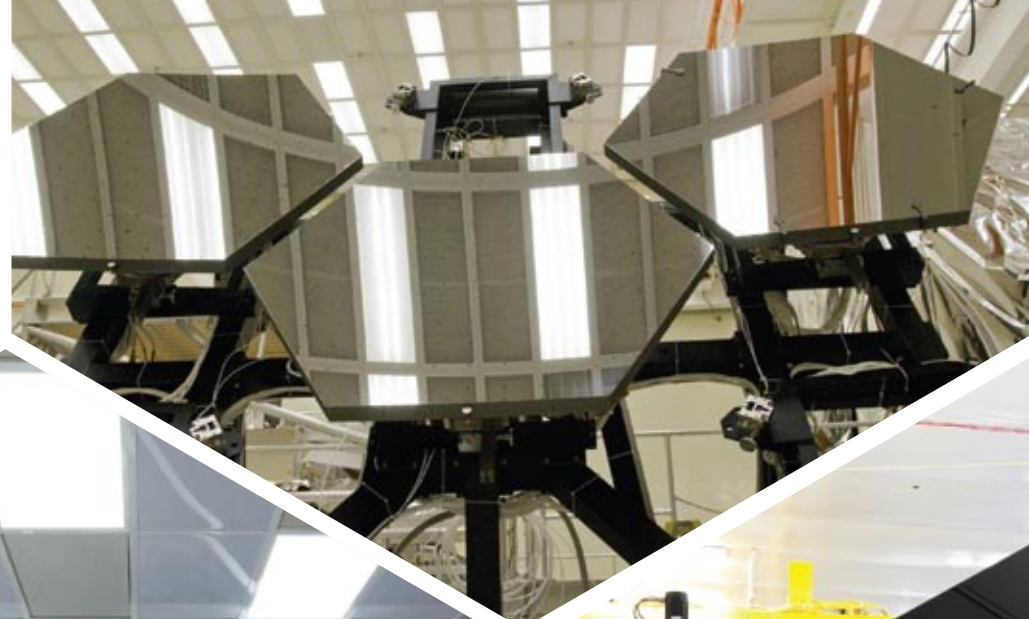
Ready to test: Segments of the James Webb Space Telescope's mirror are mounted for testing in an ultracold chamber ( top left and top right ).
