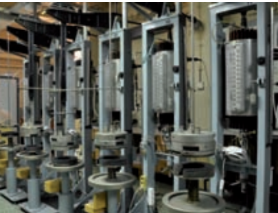
Laboratory for high-temperature creep testing.
