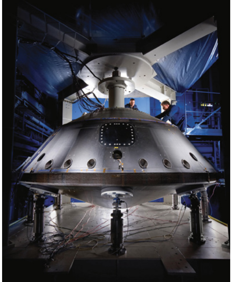
Aeroshell for the Mars Science Laboratory, scheduled to launch this month, includes an atmospheric heat shield larger than those for the Apollo capsules.
