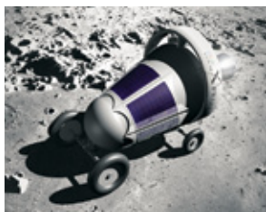
Euroluna Euroluna plans to build a four-wheeled, solar-powered rover that weighs a mere 110 pounds.
