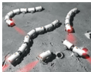
JURBAN JURBAN's small, autonomous swarm bots link up like a centipede or split up to complete different tasks.
