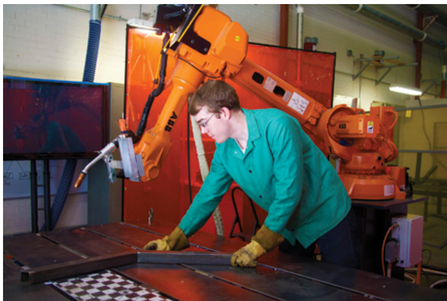
DYNAMIC DUO: Smart division of labor improves efficiency. Here the dexterous human, Carnegie Mellon engineer Michael Dawson-Haggerty, sets a piece of steel into place ( left ) before the robot makes precise welds ( right ).
