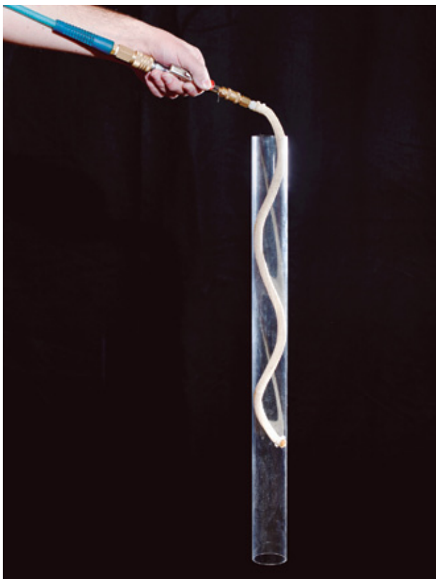
PIPE-GRIPPING HYDROSTATS such as this proof-of-concept device could eventually lead to soft, snakelike robots.
