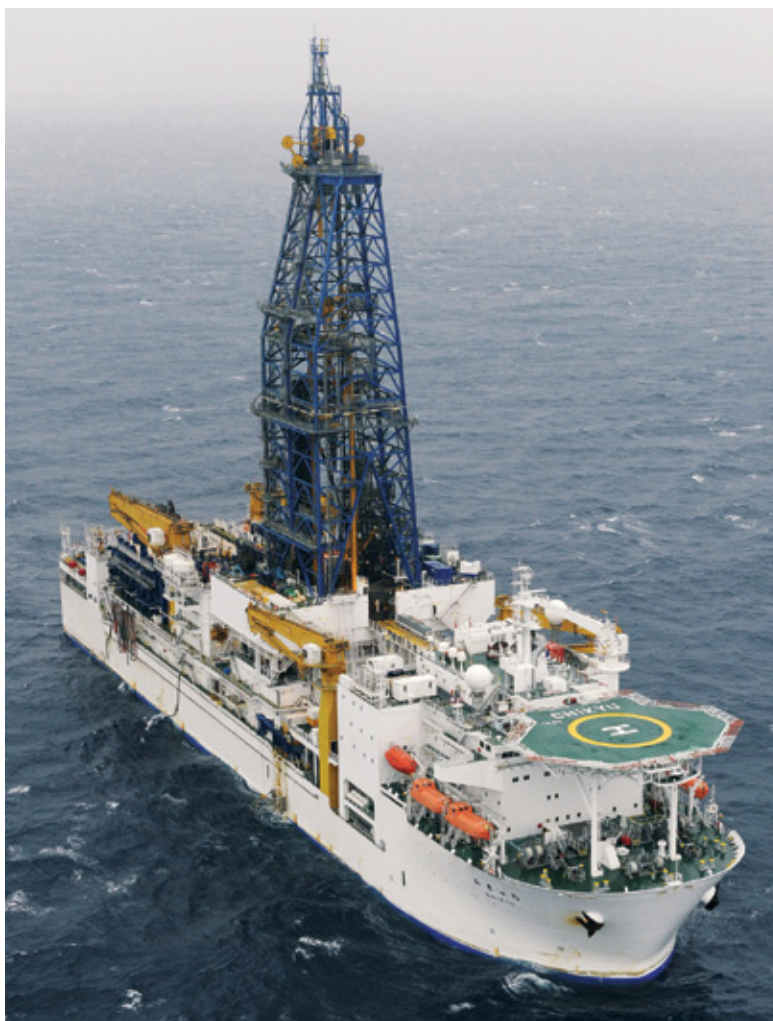
CHIKYU , a Japanese ship, prepares to drill into methane hydrates in sediments 1,000 meters below the Pacific Ocean surface.
