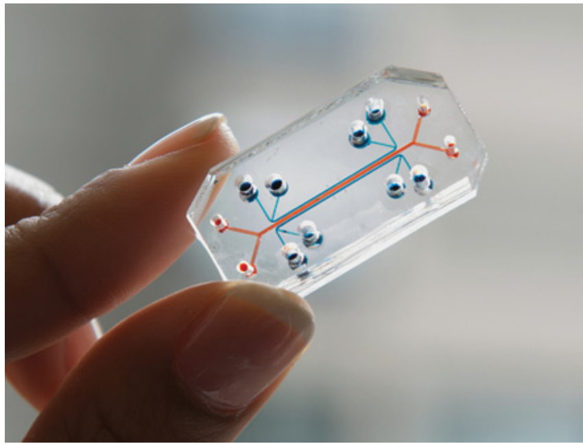
BUILDING A LUNG: When this chip created forces that mimic breathing, blood vessel and lung cells on it formed complex lung structures.
