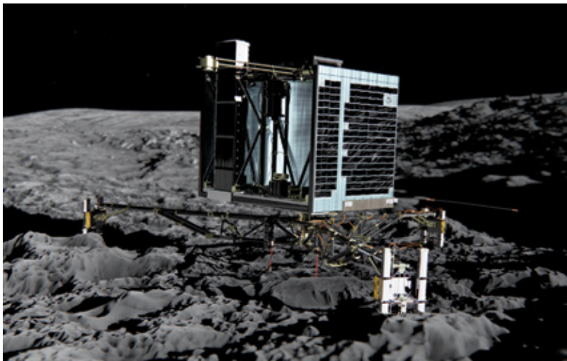
LANDING GEAR: Rosetta's Philae lander will descend to the surface of Comet 67P and attach itself with a harpoon and ice screws. There it will drill into the comet to extract samples and analyze their composition in its onboard laboratory.
