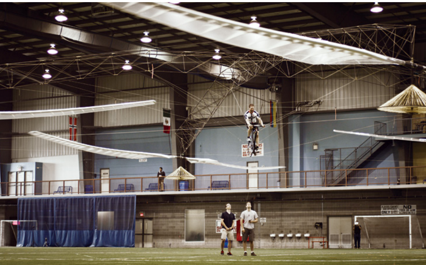
UP AND AWAY: Atlas takes off for its prizewinning flight in 2013, its four rotors carving the air in an indoor soccer stadium. Reichert, suspended below the blades and pedaling hard, kept the craft aloft and stable for just over one minute.
