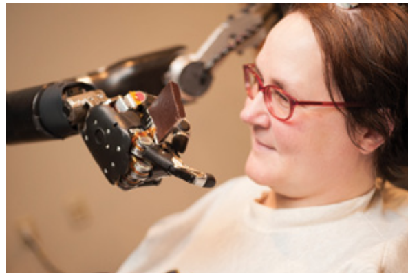
In 2012 Jan Scheuermann used her brain implant to maneuver a robotic arm toward a bar of chocolate, grasp it in its fingers, and move it to her mouth to take a bite.
