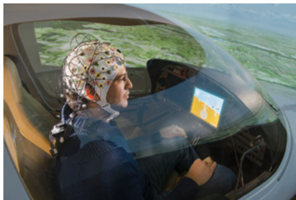
In one experiment, test pilots wore caps studded with electrodes that picked up their brain waves. So outfitted, these volunteers learned to adeptly fly—and land—simulated aircraft using their thoughts instead of their hands.
